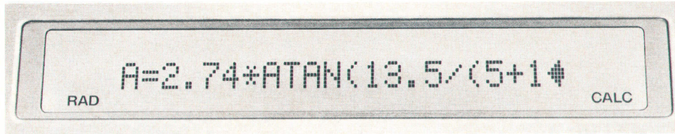
Fig. 2. The HP-71B's liquid-crystal display provides a 22-character window into a 96-character line. The pixels forming the characters can be individually read and controlled for program input and special graphics output. Display contrast and optimum viewing angle can also be adjusted for user convenience.
